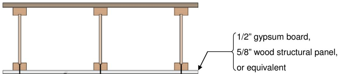
WIJMA supports the addition of a 1/2-inch gypsum wall board or 5/8-inch wood structural panel membrane, or equivalent, to the underside of floor framing systems, as required by Section R501.3 of the 2012 International Residential Code. The designer and builder shall consult with the local building department or authority having jurisdiction for specific requirements of fire protection in any building.
