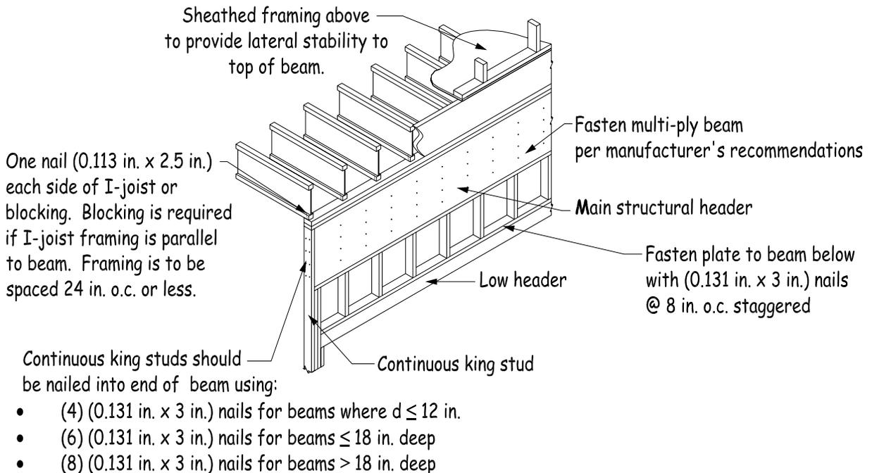
**Figure 3: Fully-Braced Alternative to Dropped Header Applications**
