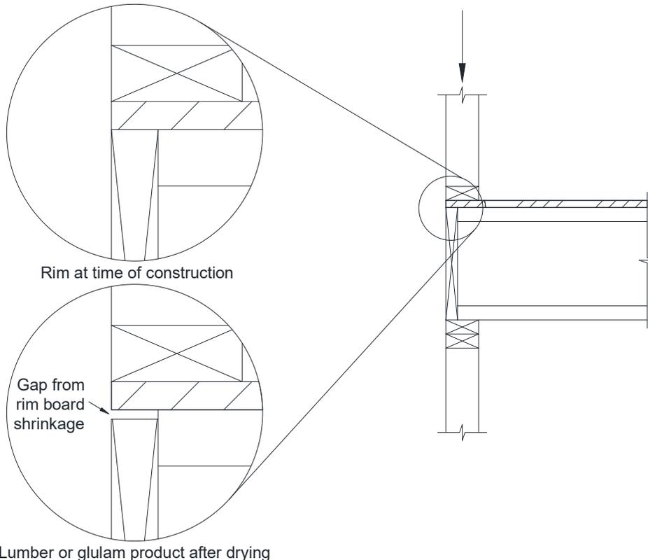
**Figure 1.** Gap caused by shrinkage of lumber or glulam product can compromise vertical load capacity leading to crushing or buckling of the I-joists and can compromise lateral load transfer capacity.
