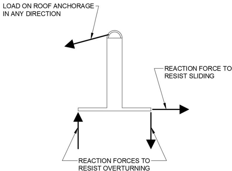
**Figure 1.** Conceptual reaction forces for anchorage. Magnitude and location of loads to be determined by fall-protection system engineer or designer of record.
