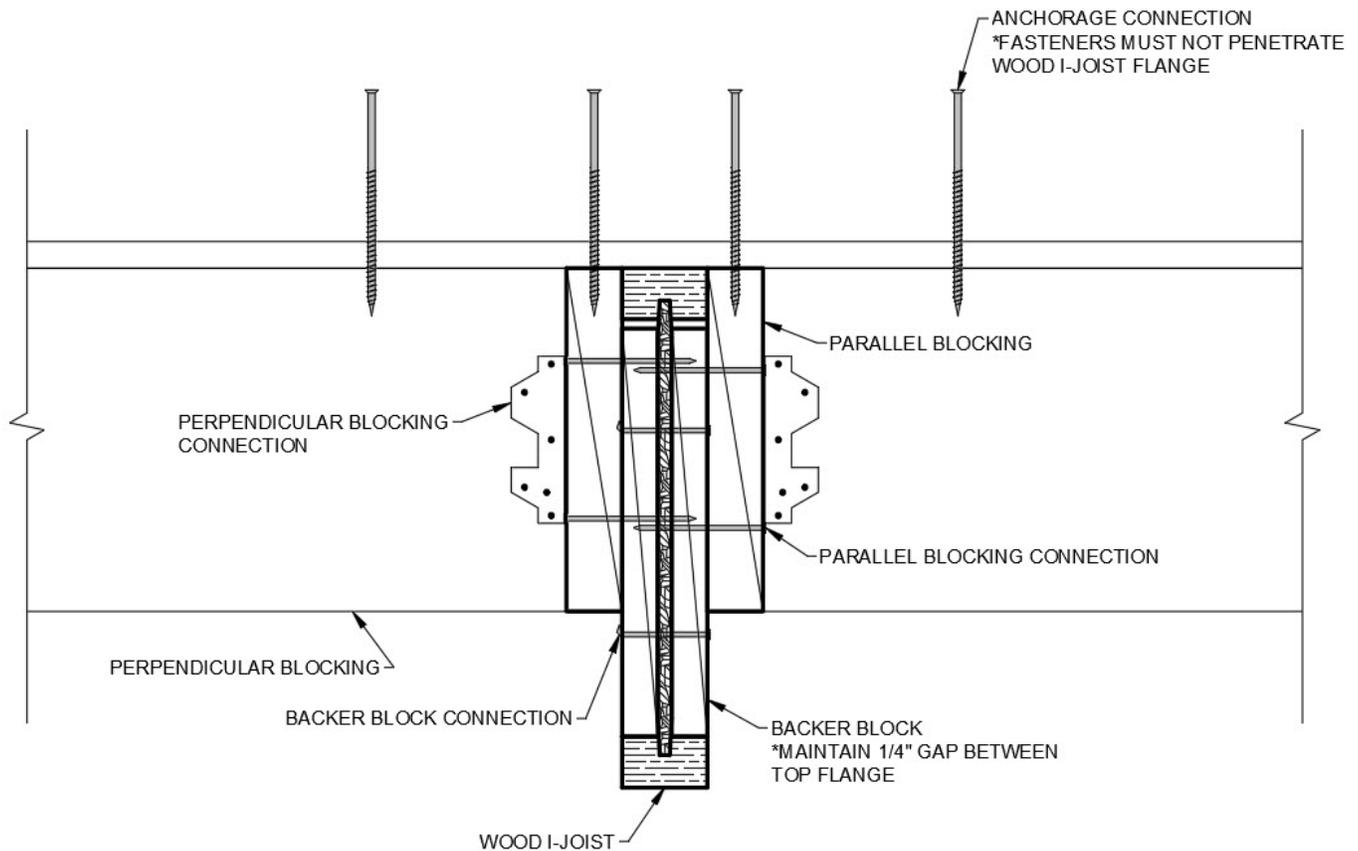
**Figure 2.** Conceptual detail for connecting anchorage to I-joist. Specific connection design and detailing to be provided by fall-protection system engineer or designer of record.
